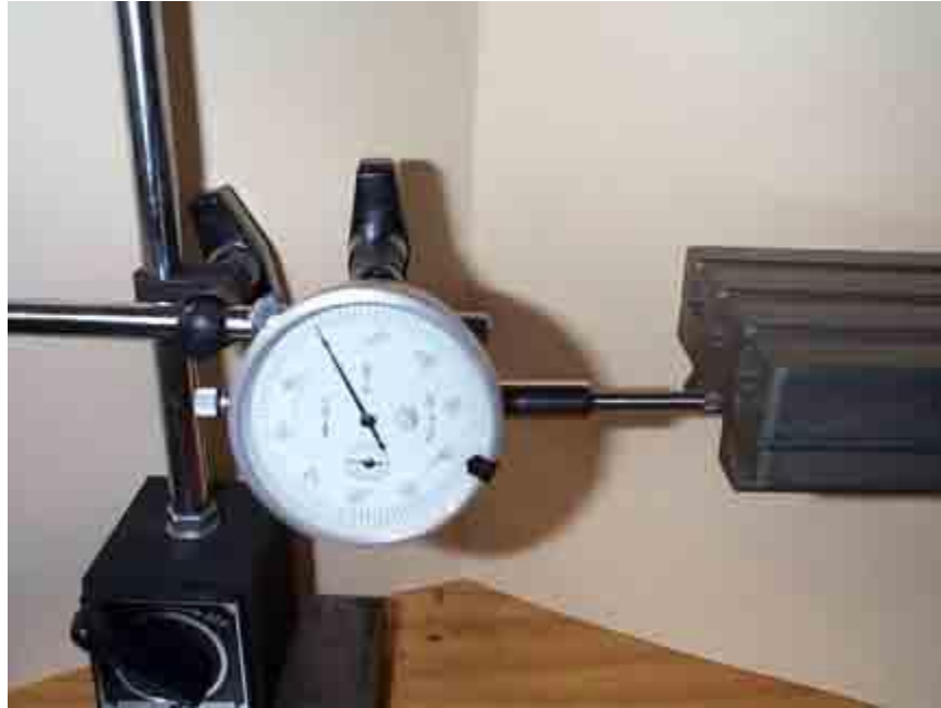
Fig. A3 - Measuring the X-axis Backlash.
