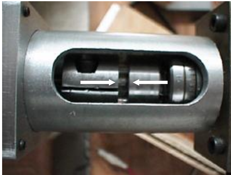
Fig. 3a - Setting the coupling Gap.
