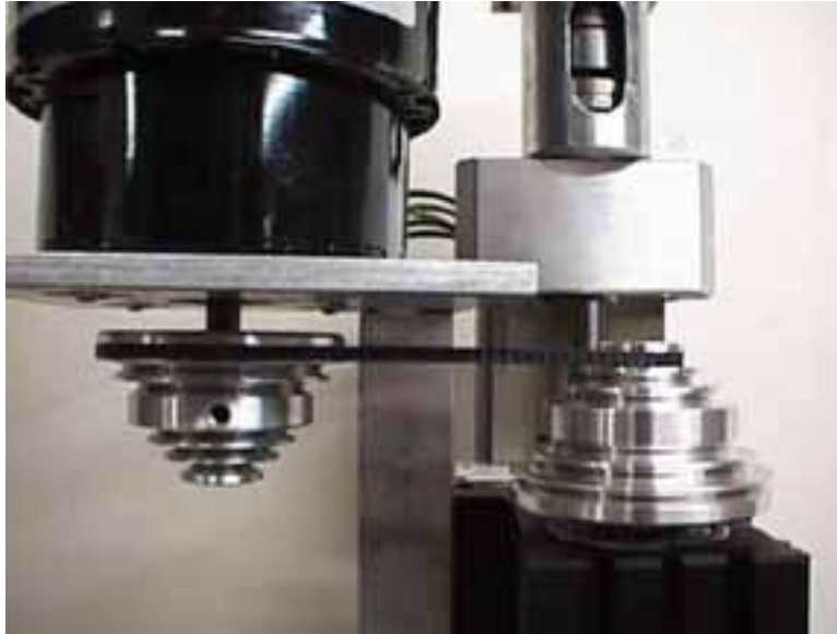
Fig. 9 - Spindle set to top speed position.
