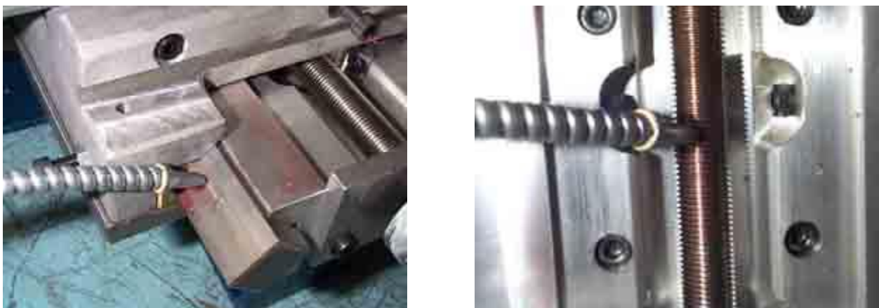
Fig. A2 - Applying Lubricant to Steel Ways and Lead Screws.
