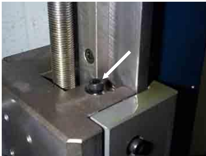
Fig. A5.1 - Box Way Brass Gib top adjustment screw.
