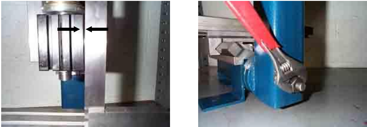
Fig. 4 - Quick squaring of Spindle to Table.
