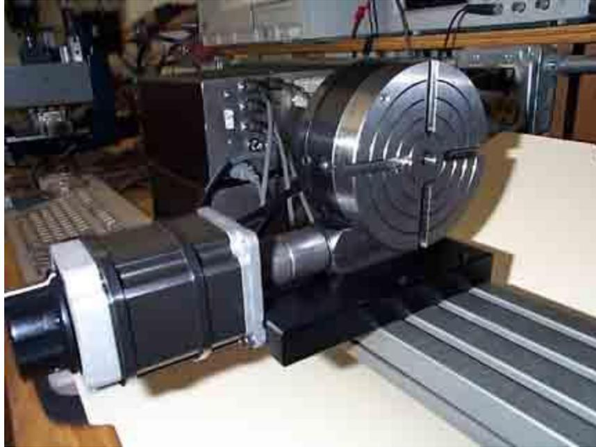
Fig. 22 - Standard mounting position of the 4<sup>th</sup> Axis Rotary Table.
