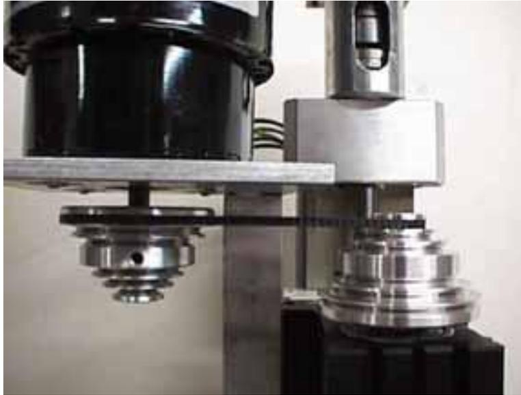
Fig. 9 - Spindle set to top speed position.
