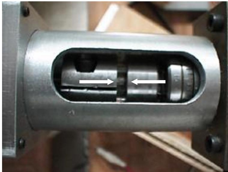
Fig. 3a - Setting the coupling Gap.
