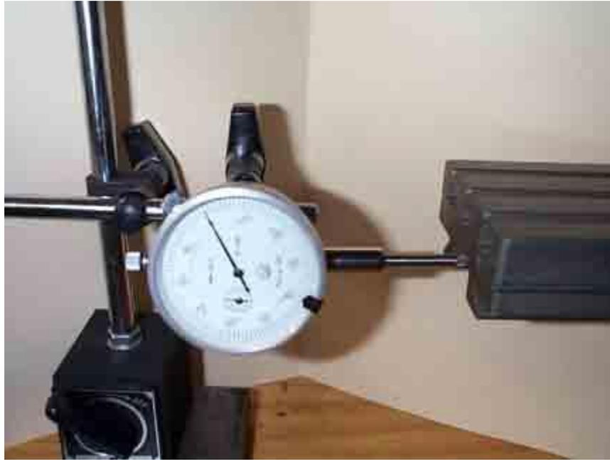
Fig. A3 - Measuring the X-axis Backlash.
