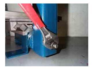
Fig. 4 - Quick squaring of Spindle to Table.
