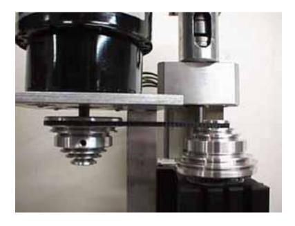
Fig. 9 - Spindle set to top speed position.
