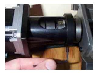
Fig. 3b - Locking the Coupling Tube in place with the Clamp Ring. Assembling the Z-axis Column:
