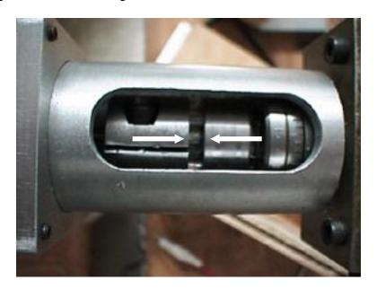
Fig. 3a - Setting the coupling Gap.
