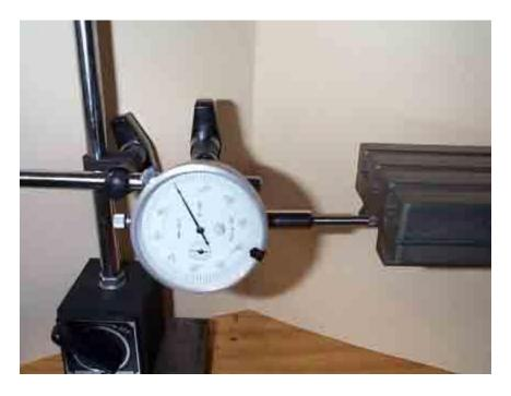
Fig. A3 - Measuring the X-axis Backlash.
