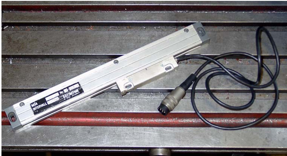
Figure 4-15: Glass Scale Encoder
