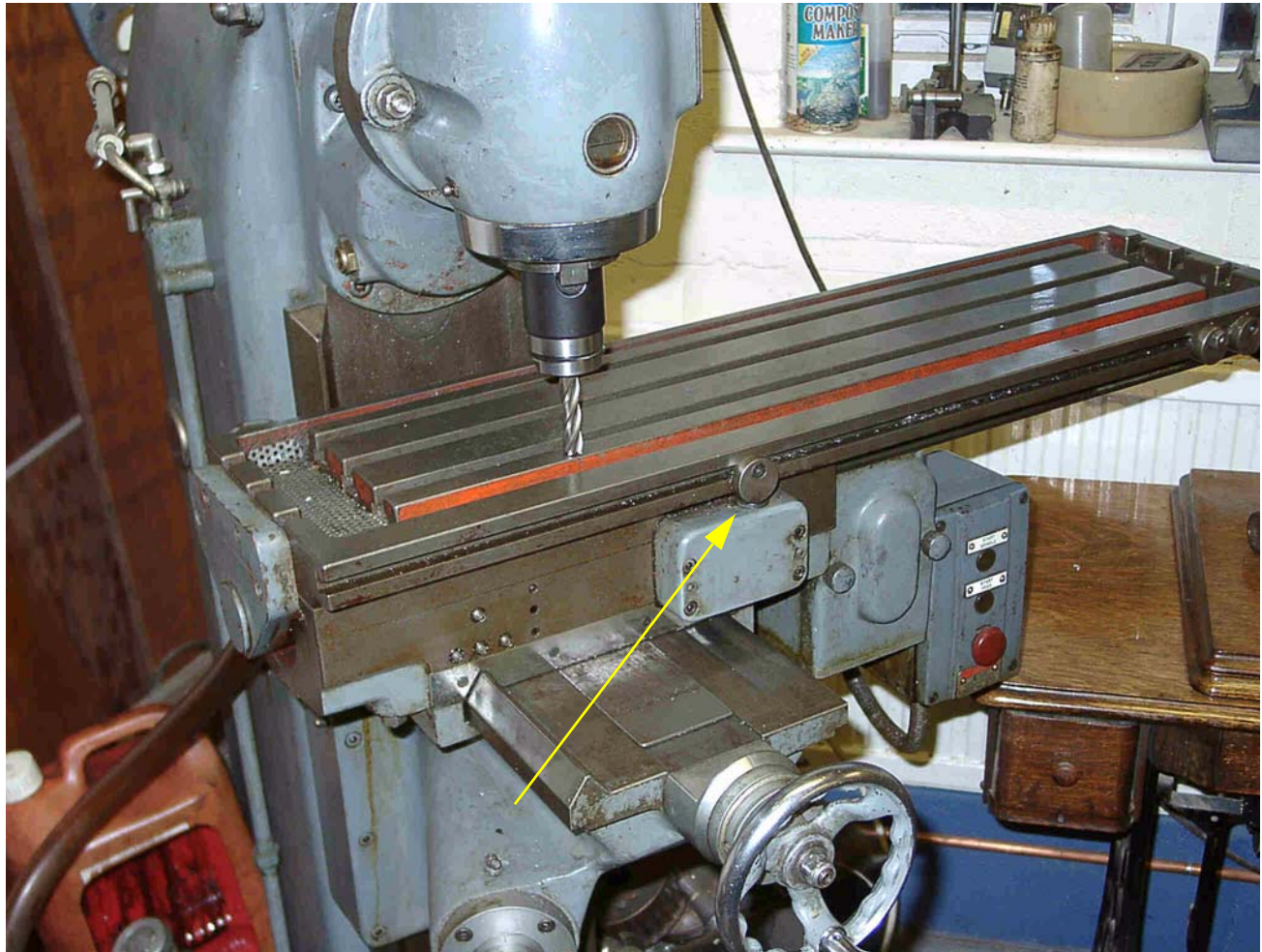
Figure 4-10: Mill with Tool at X=0, Y=0 Position (Note the Dog Is on Limit Switch)
